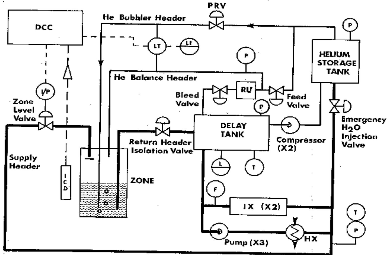
The Light Water Liquid Zone Control System - Water and Helium Circuits
