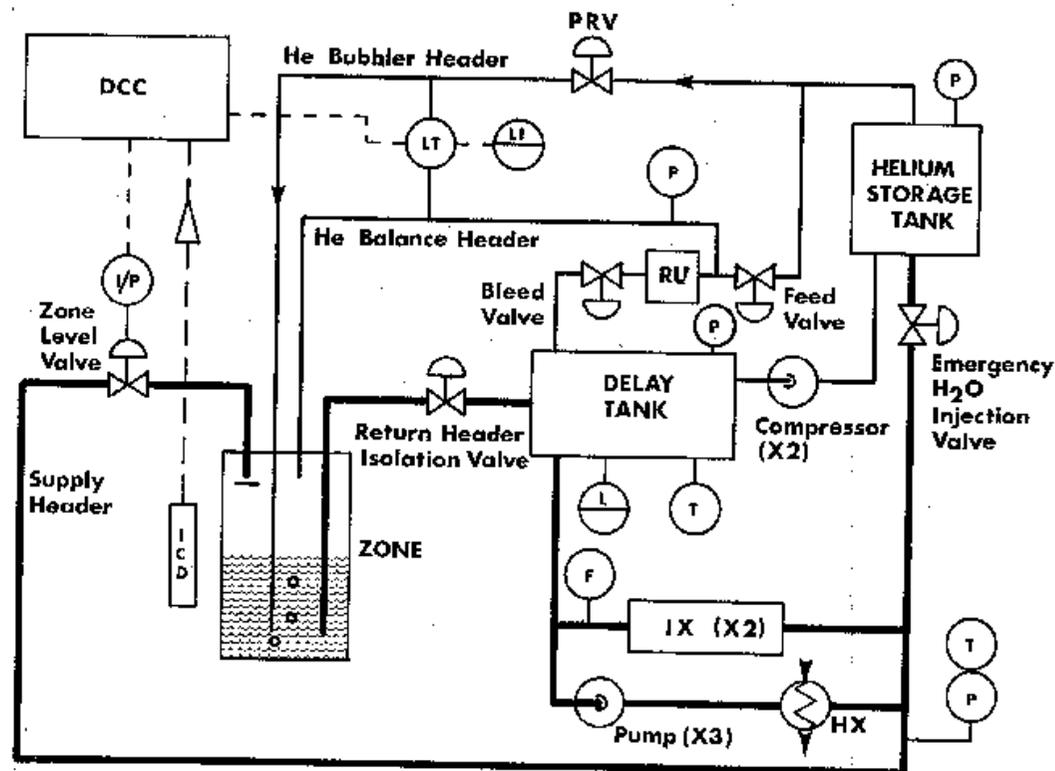
Figure 5: Zone Level Control Water and Helium Circuits.
