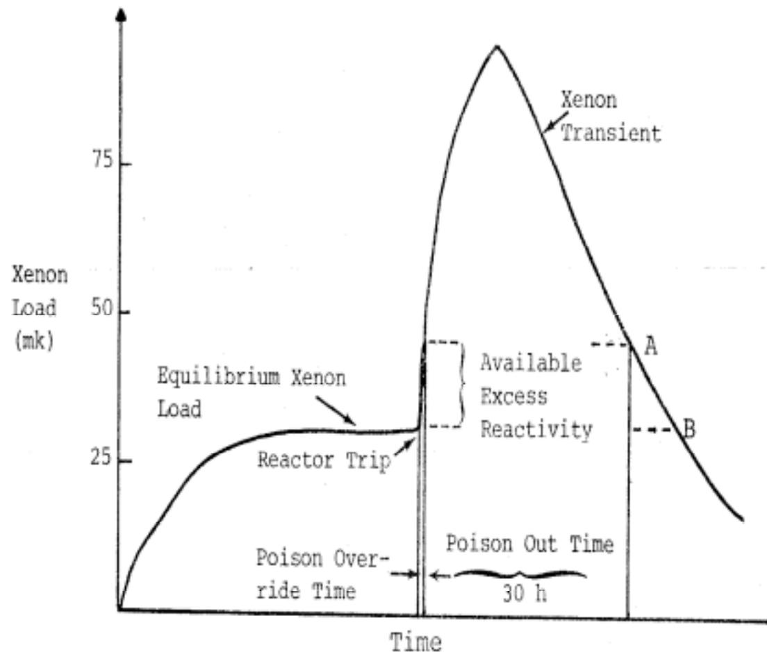
Figure 1: Xenon Load Following a Reactor Trip.
