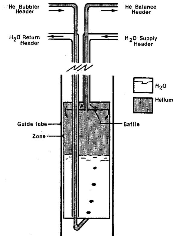
Fig 4: Typical Zone Feed Tube Connections.
