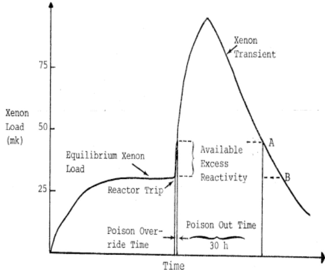
Figure 1: Xenon Load Following a Reactor Trip.
