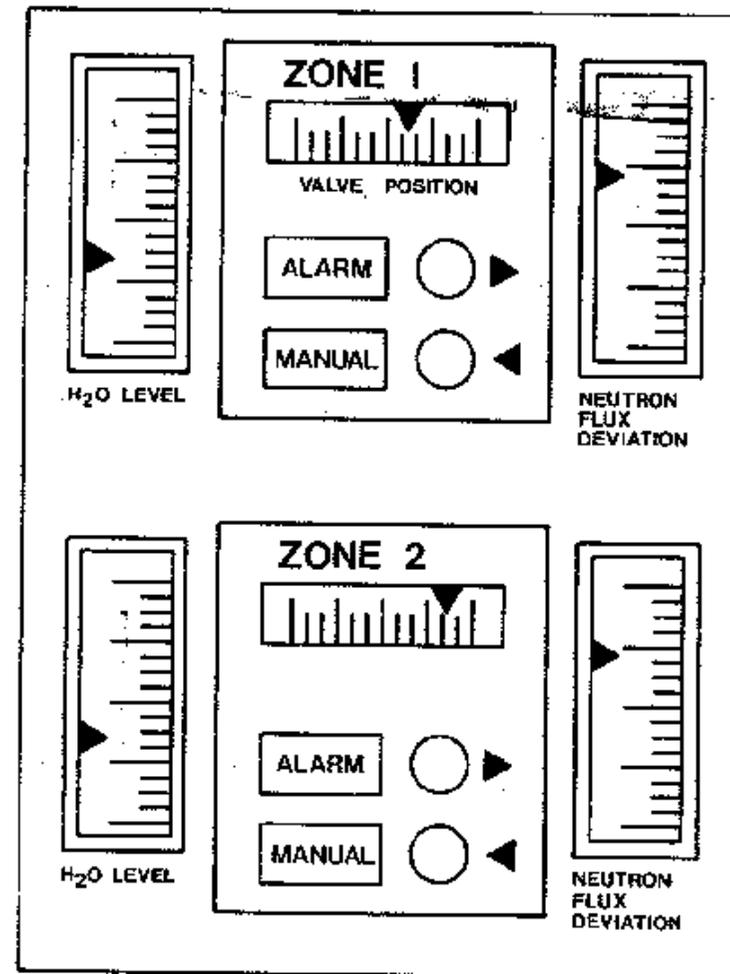
Figure 6: Zone Control Panel Manual Loading Station.
